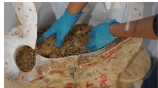
Figure 18. *Lingzhi* grow mould made of fiberglass resin.
